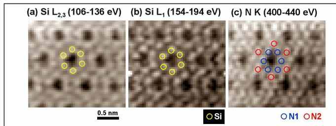
Figure 6: Characteristic signal maps of the  $\text{Si L}_{2,3}$  (a),  $\text{Si L}_1$  (b) and  $\text{N K}$  edges (c) modified from the maps in Figure 5 by applying the Wiener filter, which is available in the HREM-Filters Pro plug-ins. The Si positions and two types of N positions (denoted as N1 and N2) are overlaid in either the Si maps or the N map, respectively.
