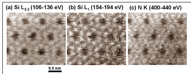
Figure 5: Characteristic signal maps of the  $\text{Si L}_{2,3}$  (a),  $\text{Si L}_1$  (b) and  $\text{N K}$  edges (c) obtained from the PCA-reconstructed Si dataset with background subtraction.
