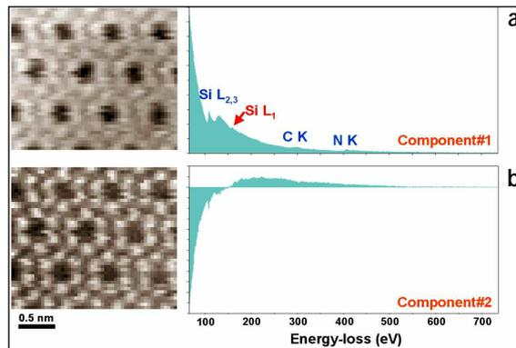
An SI dataset acquired as a 3D data cube with the spatial dimensions  $(x, y)$  and the spectral (energy channel) dimension  $E$  can be converted into a 2D data matrix  $\mathbf{D}_{((x,y),E)}$ . By applying PCA, this matrix can be decomposed as:
