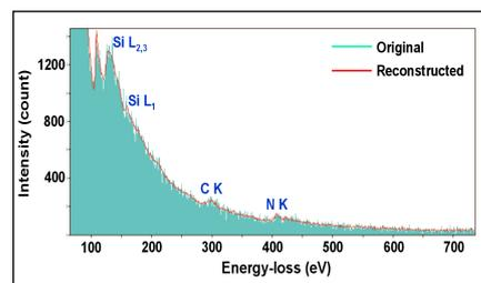
Figure 4: Comparison of EELS spectra at a single pixel extracted from the original and PCA-reconstructed SI datasets.
